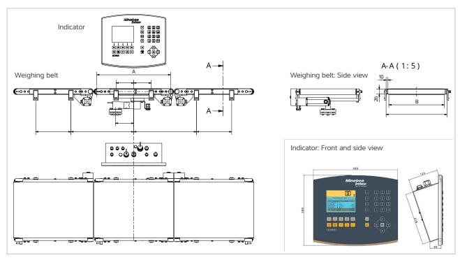
**Legend** A: Centre-to-centre distance of the conveyor belts B: Conveyor belt width
