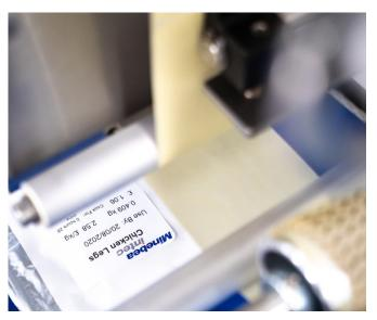
The WPL-A convinces with high-speed printing of up to 125 labels per minute, made possible using advanced print compression technologies.
